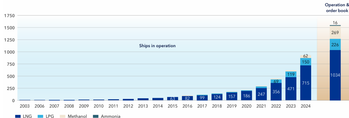
Growth of the number of ships capable of using selected alternative fuels, excluding LNG carriers, as of May 2024
